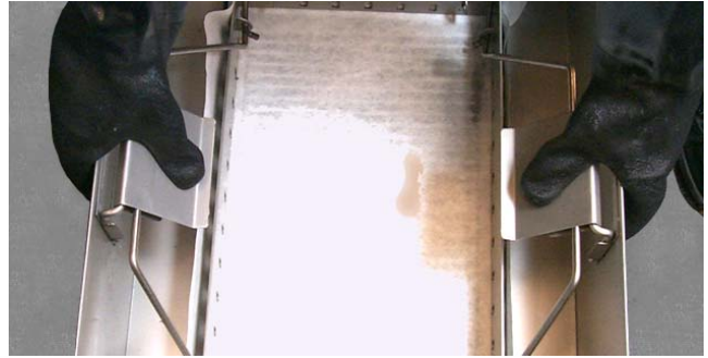
Locking hold-down ring in place.
